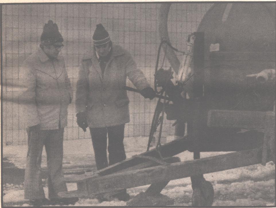
Above: Dr. Satish Negi, Research Associate and Faculty Lecturer, on the left, and Dr. Edward McKyes, Associate Professor and Chairman, Department of Agricultural Engineering, inspect the subsurface liquid manure injector which they designed and mounted on one of the Macdonald College farm's manure tank wagons.
