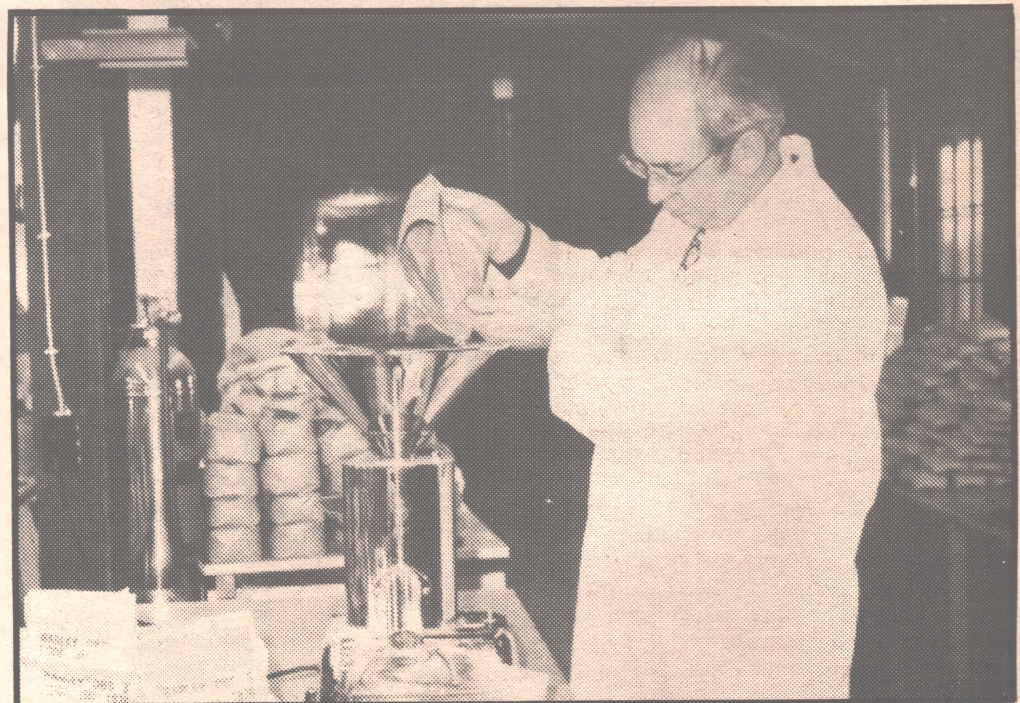
Dr. H.R. Klinck, from the Plant Science Department, pouring grain into a precision grain divider at the Emile A. Lods Agronomy Research Center.
