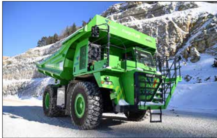
The eDumper is a 45-ton dump truck that never uses more energy than it generates while going up and down its mountainous worksite. (Courtesy: eMining Switzerland)
