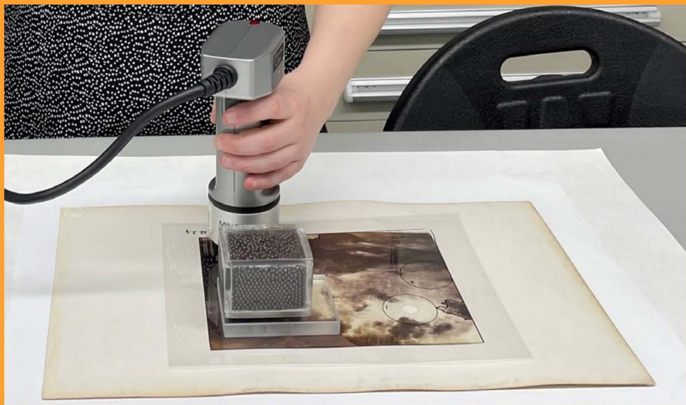
Colorimetry measurements in progress on an Alexander Henderson photograph, MP-1976.122.2.4.
