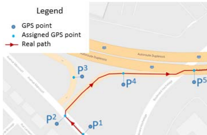
Figure 1. Incorrect assignment of point P^3 under the point-to-curve technique
