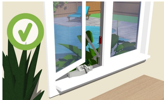
Window opening restrictor.
