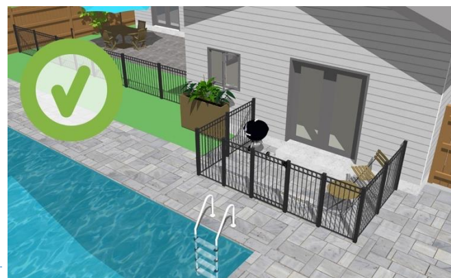
Patio door surrounded by a fence to prevent direct access inside the pool enclosure.
