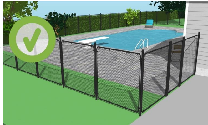
Example of a chain-link fence with a mesh that is less than 30 mm wide.
