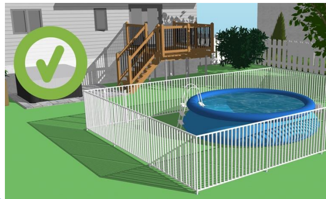
Example of a portable pool less than 1.4 m high to be surrounded by an enclosure.
