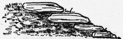
EMBEDDING ROCKS (GIVE SLIGHT TILT INTO SLOPE)
