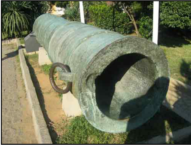
Figure 2.5: Cannon used in the siege of Constantinople, 4.25 m long, 63 cm diam., and 14 cm thick, used to throw stone balls 285 kg [Military Museum in İstanbul]. Photo by Nadia Habashi, 2006.
