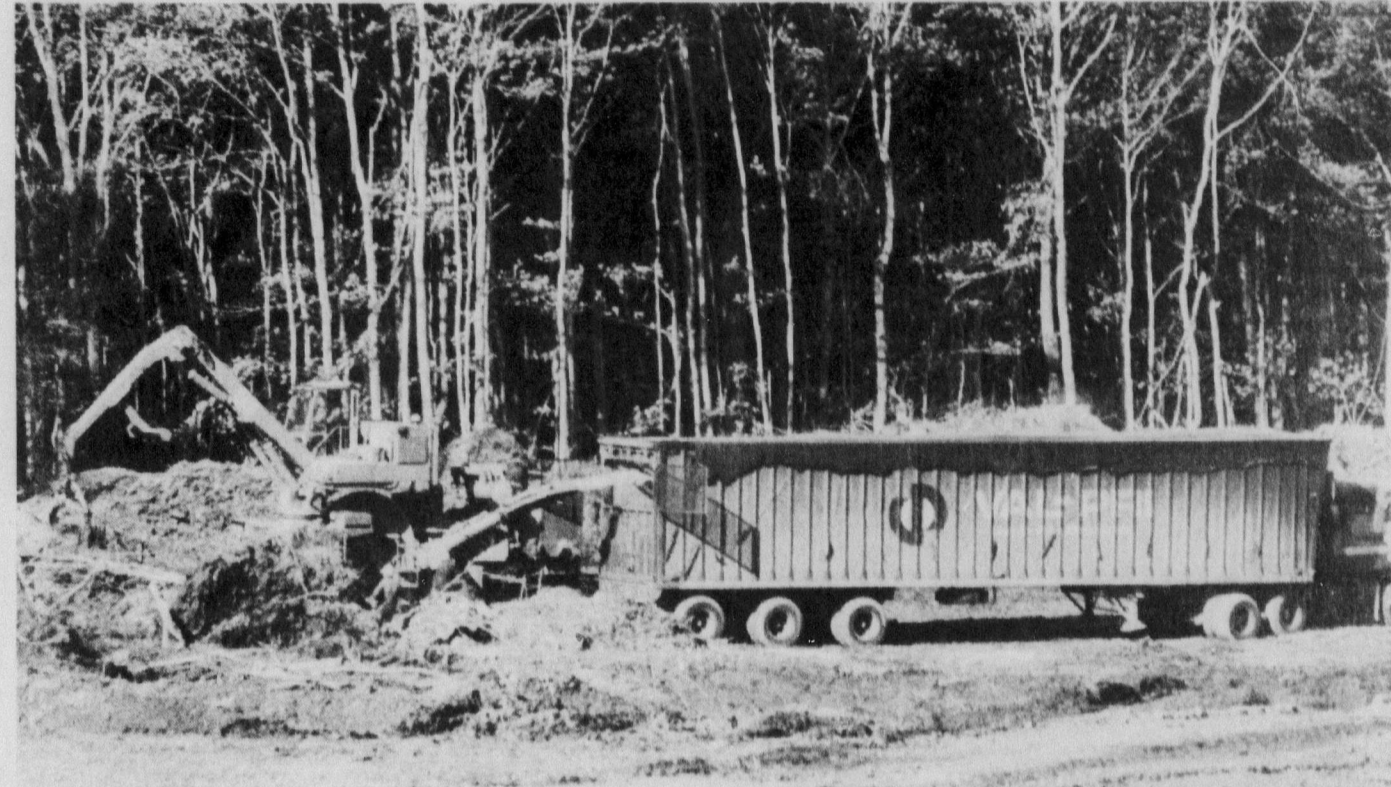
The chipper uses a giant arm to push whole trees into its maw, then blows the chipped hardwood into one of a proposed 30 trucks a day. Local residents have complained about the chipper's high-pitched whine and the heavy truck traffic, but the report downplays its importance.
