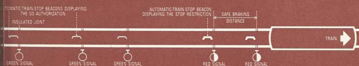
AUTOMATIC-BLOCK SIGNALING FEATURING THE BUFFER ZONE AND DISCRETE CONTROL OF TRAIN INTERSPACING
