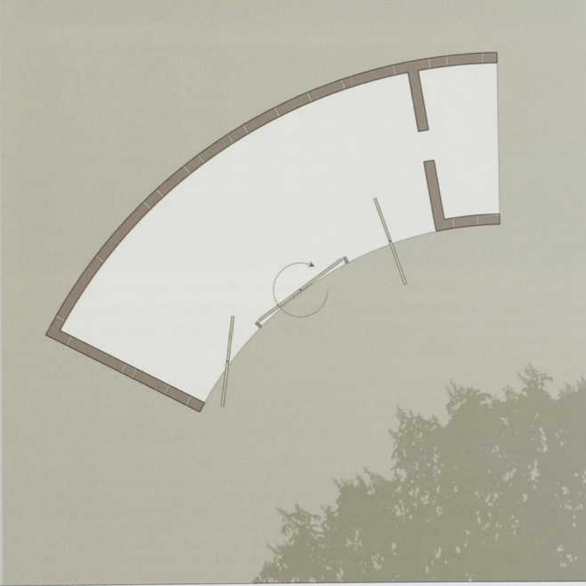
Plan of a typical rammed earth module The pivoting chalkboard panels allow interior and exterior lessons.
