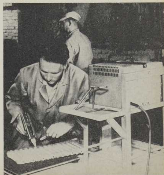
FIG. 6—ULTRASONIC RECTIFICATION OF SURFACE FAULTS ON ALUMINUM-ALLOY CASTING.
