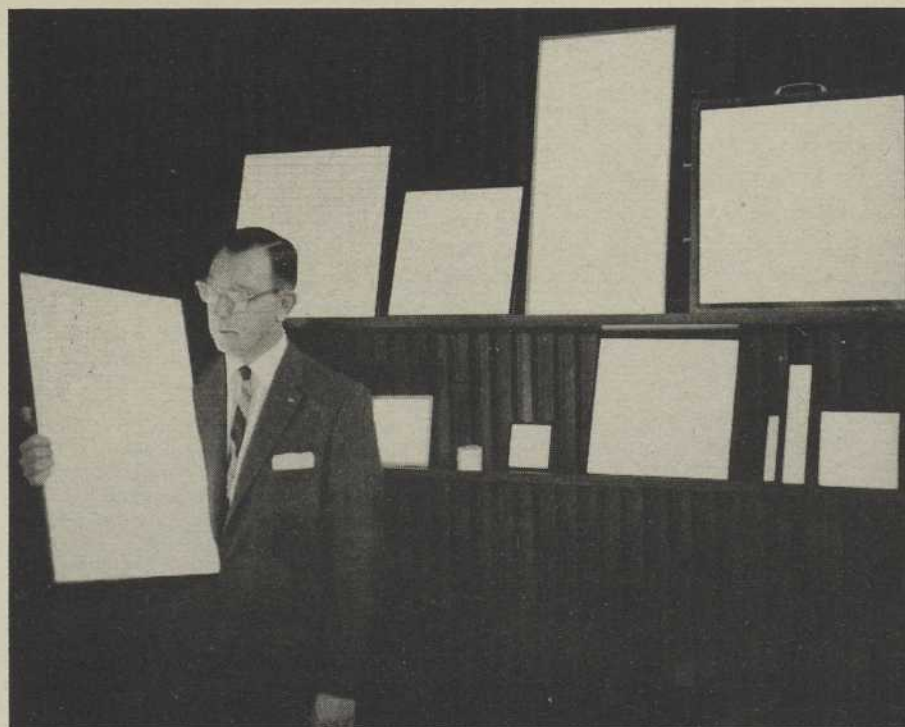
Electroluminescent Lamps are glass sheets having an electrical conductive coating and phosphor layer, to which voltage is applied to produce light. Resembling glass panes, the lamps produce diffused light with little electricity. Many uses include shelf lights, signs, clock faces, and decorative lighting. Available in green, yellow and blue, they come in various sizes. (Westinghouse Electric Corporation, Lamp Div., Bloomfield, N.J.)
