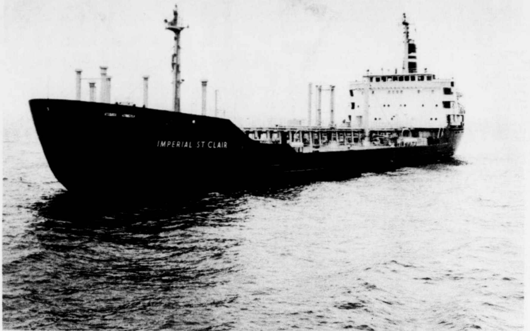
NEW TANKER — The new 12,600-ton Imperial Oil tanker, Imperial St. Clair, has successfully passed her trials and will go into service in mid-April, operating out of Sarnia and Montreal. The 435-foot vessel has an ice-strengthened bow, stern and rudder, enabling her to operate for an extended shipping season on the Great Lakes and St. Lawrence River and also to undertake summer supply voyages to the Arctic. A special feature of the new tanker is a clean ballast system which will obviate the need for additional water to be taken into product tanks except under severe weather conditions.
