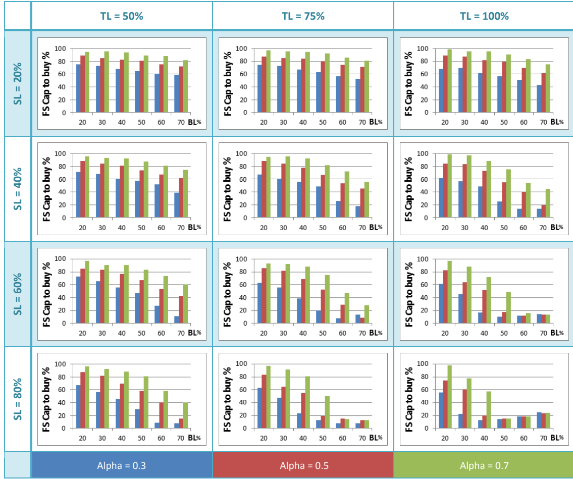
Figure 5.16: Percentage of estimated capacity that should be booked at the first stage for instance set T5, availability class AV1 and uniform losses.
