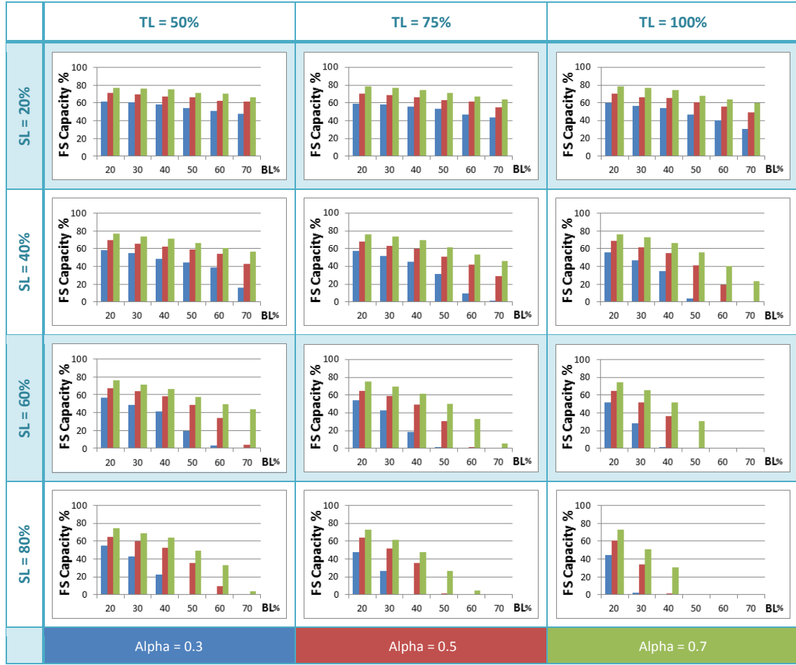
Figure 5.7: Percentage of capacity booked at the first stage for instance set T3, availability class AV2 and uniform losses.
