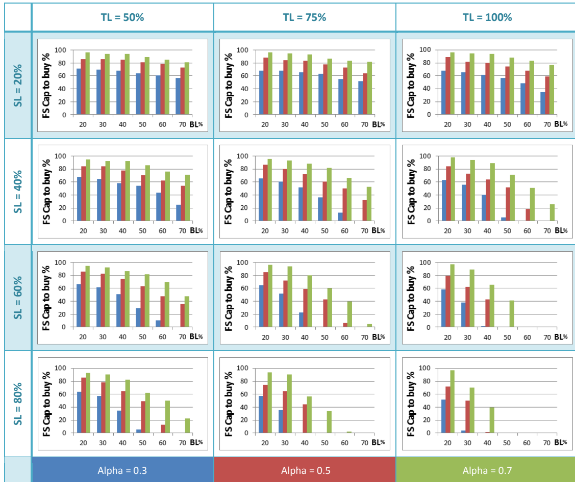
Figure 5.21: Percentage of estimated capacity that should be booked at the first stage for instance set T5, availability class AV2 and uniform losses.
