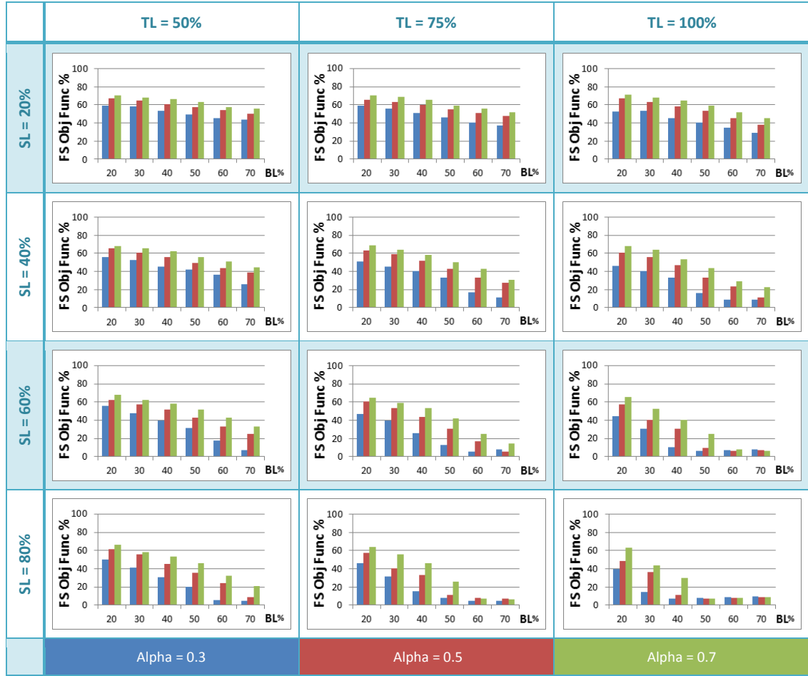
Figure 5.13: Percentage of objective function value achieved at the first stage for instance set T5, availability class AV1 and uniform losses.
