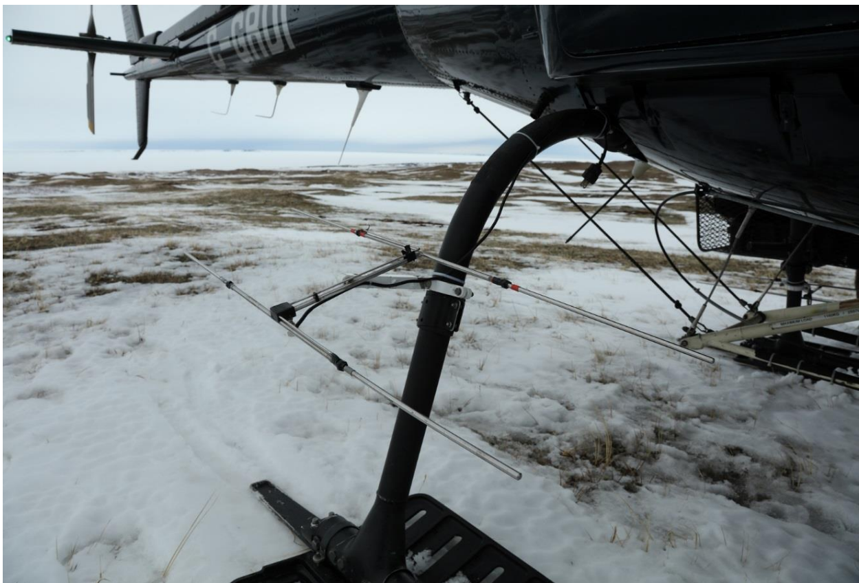
Figure 3: Example of one of the three type “H” directional antennas attached to the helicopter’s skids using a fastener approved by Transport Canada and connected by means of a coaxial cable to the VHF telemetry system.
