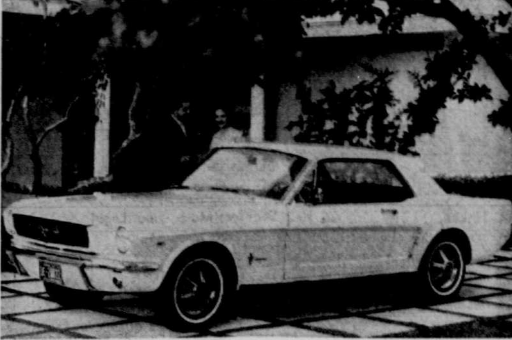
This is Ford of Canada's new Mustang. The low, sleek automobile is designed as a family sports car, with bucket seats in front, room for two adults in the back and ample trunk space. Two body styles are offered: a hardtop coupe and a convertible. Four engines, ranging in power from a 101 h.p. six, 164 h.p. V-8, 210 h.p. V-8 to a 271 h.p. V-8 will be available, with 3-speed manual, 4-speed manual and automatic transmissions. Sports car drivers will be able to order a "special handling package" for maximum roadability. Luxury options include power assists, vinyl-covered roof, tinted glass, console and air conditioning.
