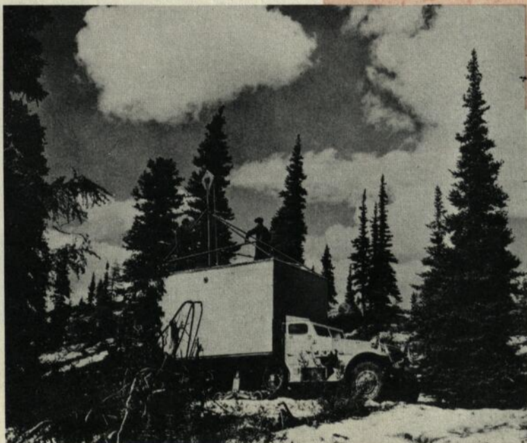
Portable drills mounted on modified trucks were used for exploration where the terrain permitted. The first drill like this was used in 1947. Three more followed in 1948.
