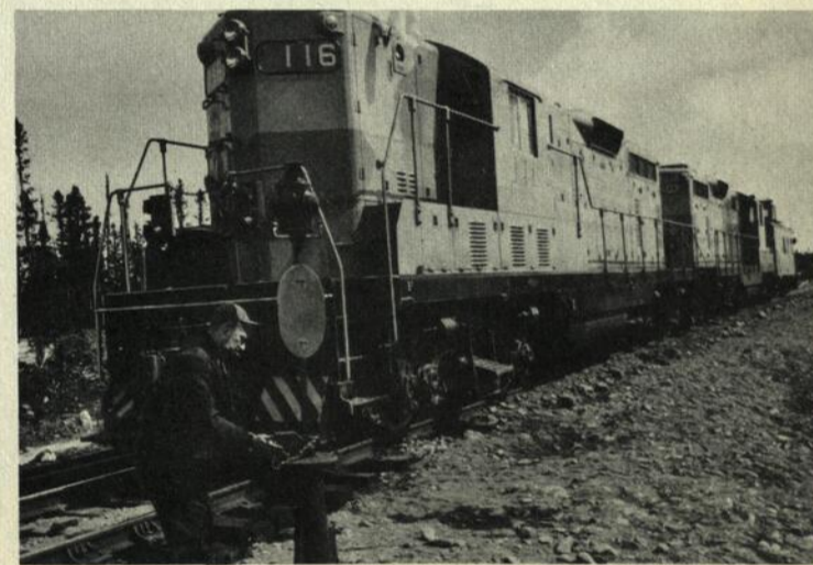
Hand switches like this lead to temporary pit spurs. Power-operated switches are used on main line sidings.
