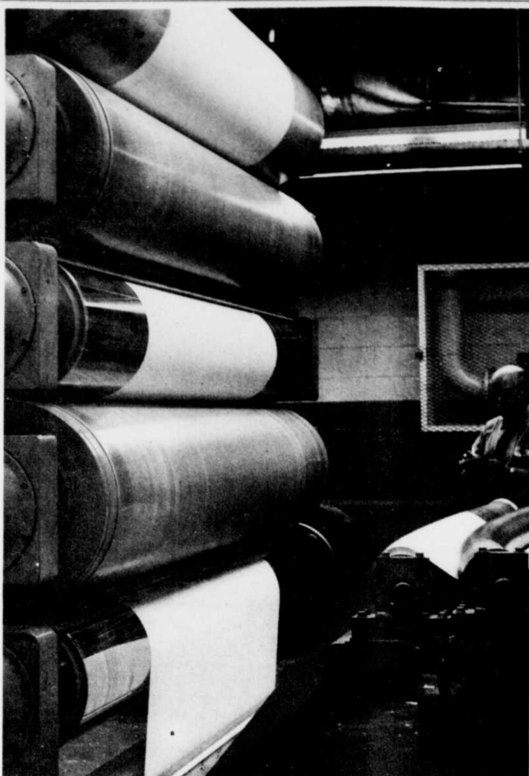
An enormous five-bowl calendar unit, weighing 60 tons, has been installed at the Dominion Textile Print Works in Magog at a cost of $1,000,000. Foreman Elie Rancourt controls the machine's efficiency. Story and picture on Page 5.
