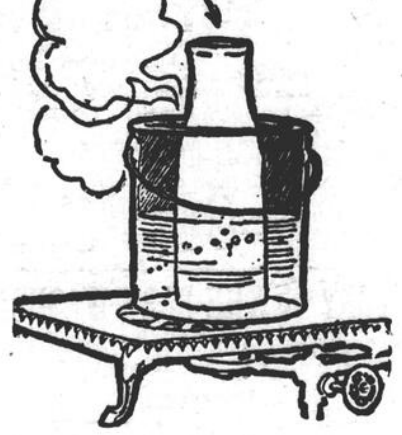
EXPLANATION OF METHOD BELOW: MILK BOTTLE (A) IN TIN PAIL (B) IN CRANKED BOX (C). (C) IS AIR SPACE BETWEEN MILK AND CILINDER. (B) IS SAWDUST PADDED OUTSIDE OF CILINDER TO THE TOP OF BOX (C). (A) IS COVER, SHOWING HOW THE PASTEURIZER IS PLACED TO BOIL. SIDE.
