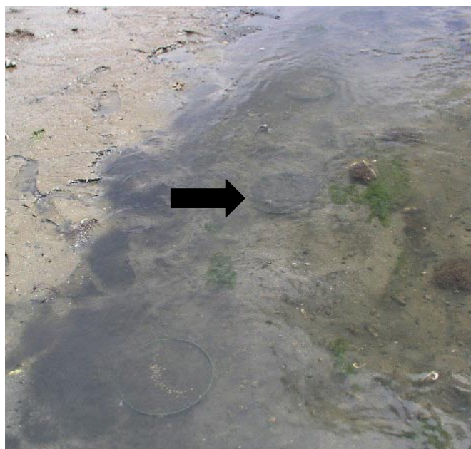
Figure 3. Cylinders buried in substrate and filled with substrate were used to monitor clam survival and growth in units with predator exclusion netting and without netting.
