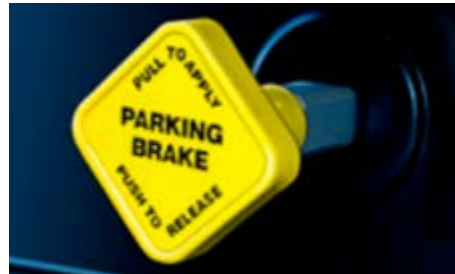
FIGURE 65 | Parking brake air supply control
