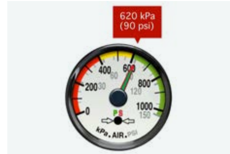
FIGURE 68 | Pressure gauge indicating a pressure of 620 kPa (90 psi)
