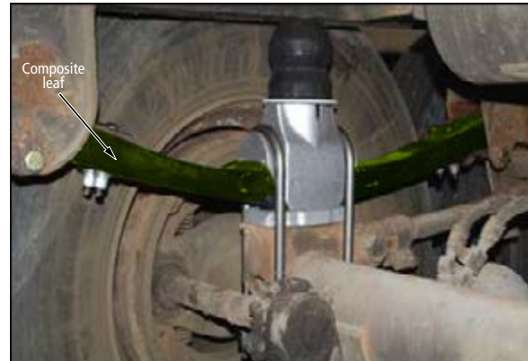
FIGURE 53 | Composite leaf spring
