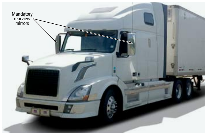
FIGURE 42 | Rearview mirrors on a truck
