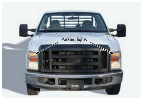
FIGURE 36 | Front parking lights of a vehicle that is 2.03 m wide or less.
