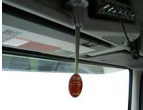
FIGURE 67 | Visual warning device (wig wag)
