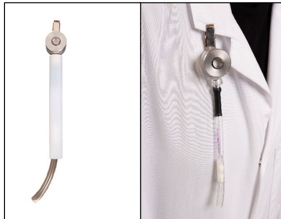
Figure 34. IFV Pro Sampler de SKC
