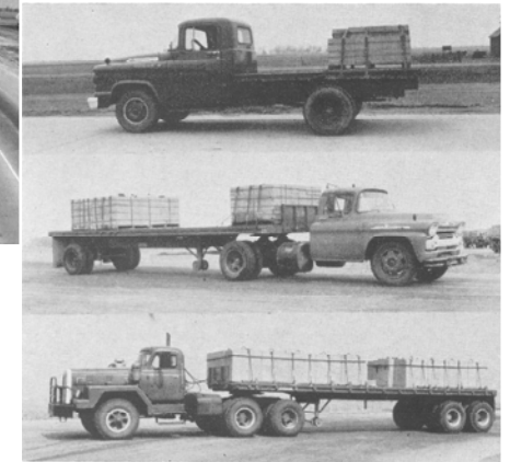
Figure 23. Test vehicles, showing typical axle arrangements and loadings.
