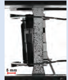
Figure 2. Experimental setup featuring extensometer and speckle pattern on the sample
