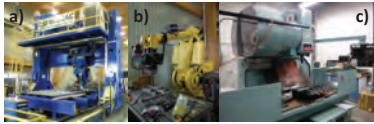
Figure 2 – Welding equipment a) MTI gantry b) Fanuc robot M-900/600IA c) Millac 5VA universal milling machine
