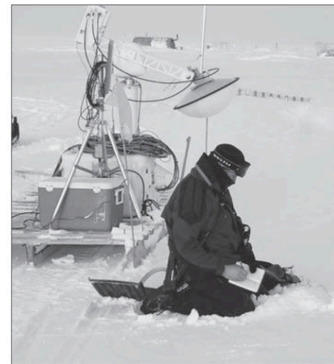
Doing snow measurements affecting the radar signal (radar in the back) (Franklin Bay, Nunavut).
