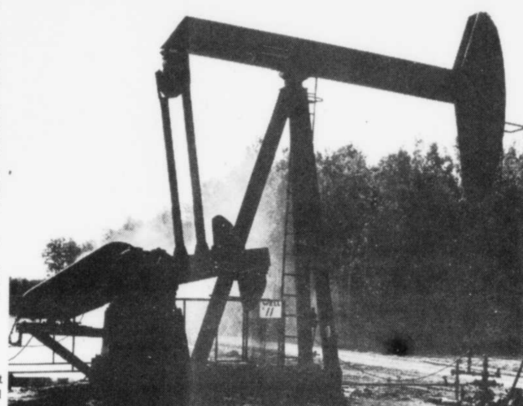
HEAVY OIL EXTRACTION — This "horsehead" pump near Cold Lake in Alberta is part of a field demonstration research program to find ways of producing oil from one of Canada's major petroleum reservoirs. Second only to the Athabasca tar sands in size, the Cold Lake oil sands hold oil too thick to be pumped
