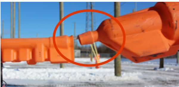
Part of conductor exposed due to faulty interlocking of conductor covers
