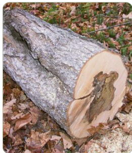
Figure 39 — Fente spiralee profonde (bourrelet)
