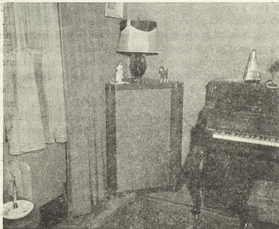
A corner loud speaker cabinet with an 8-inch speaker for a small room
