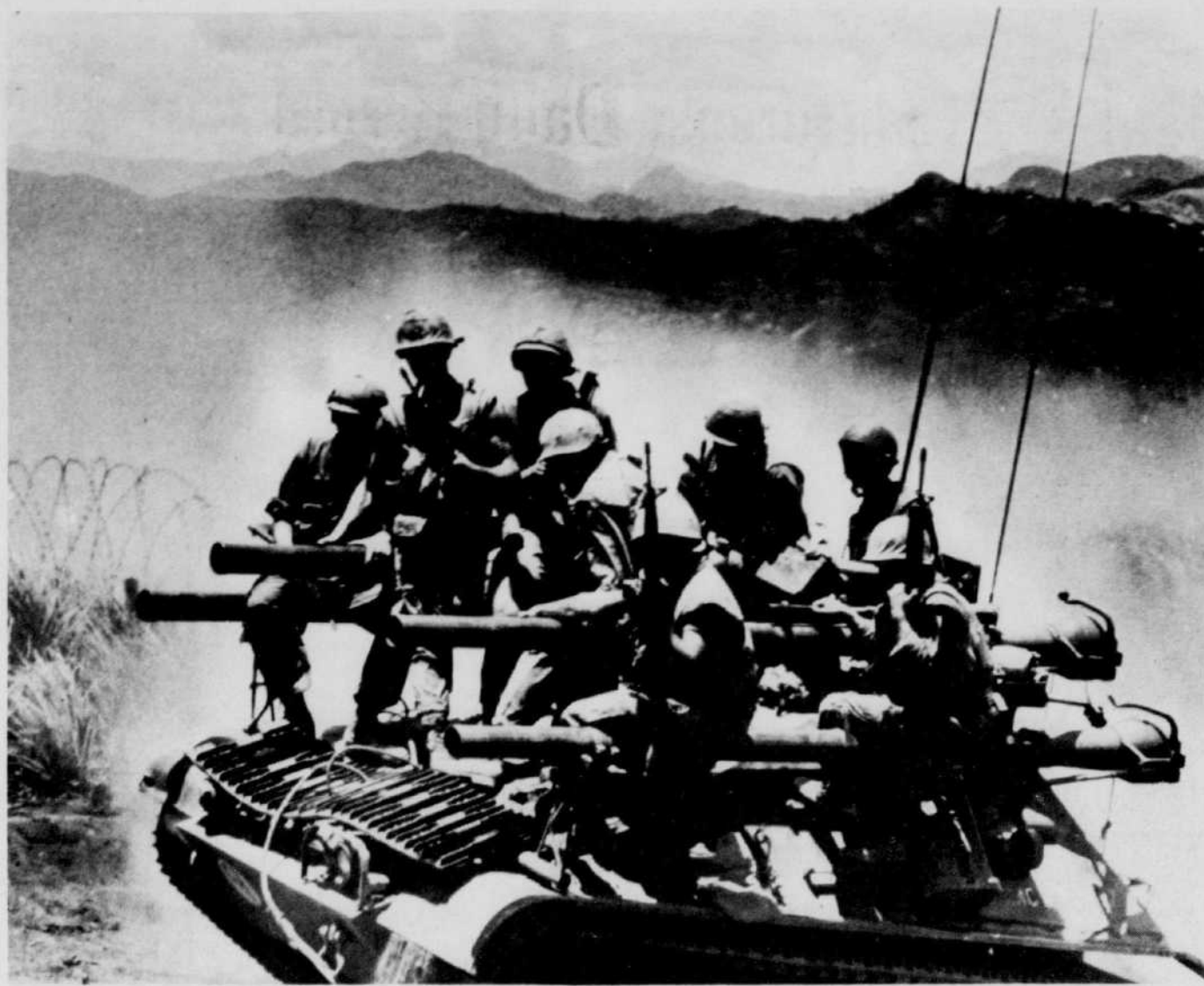
HIT THE DUSTY TRAIL — Marines of the first battalion 9th Marines ride an ONTOS, a light weight tank-like vehicle carrying four 1.6mm recoilless
