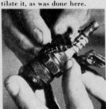
What do you do when the spark plug insulator breaks? Wrap it with some plastic tape and keep on driving . . . but probably not for long.
