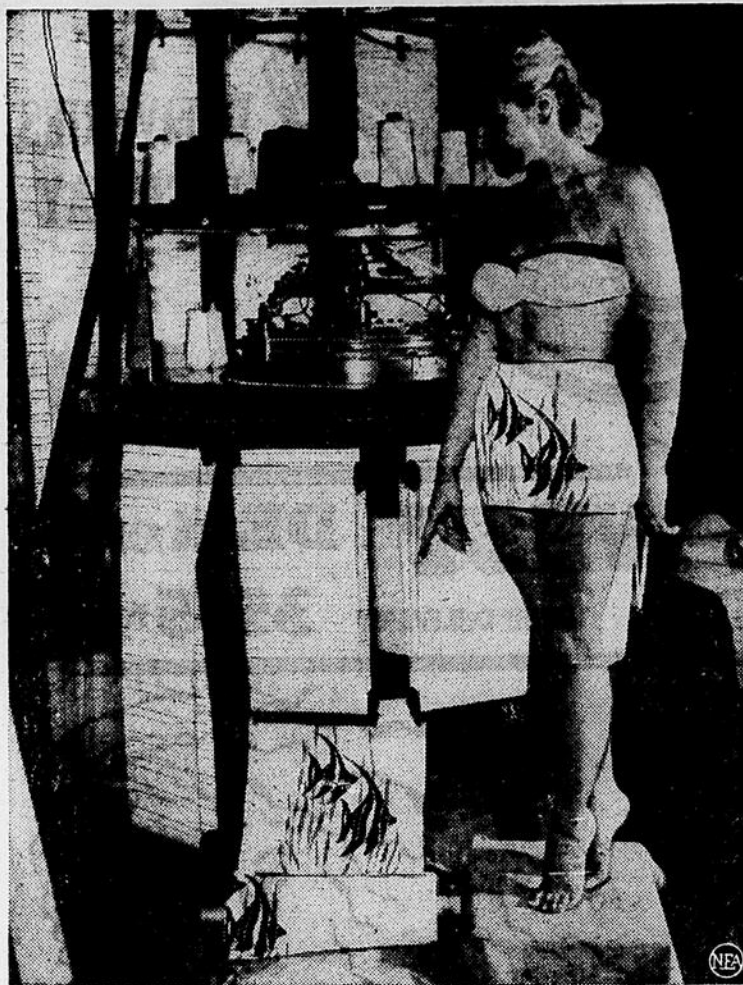
Anyone who would rather think of sun and balmy breezes instead of slush and snow will be glad to hear that knitting mills are clicking 24 hours a day to meet next season's demand for bathing suits. On the complicated automatic machine above in Los Angeles, nine patterns, resembling rolls of an old-fashioned player piano, are needed to guide the thousands of needles turning out the new Catalina angel fish design. Bette Stewart models a completed suit as the cloth leaves the bottom of the machine.
