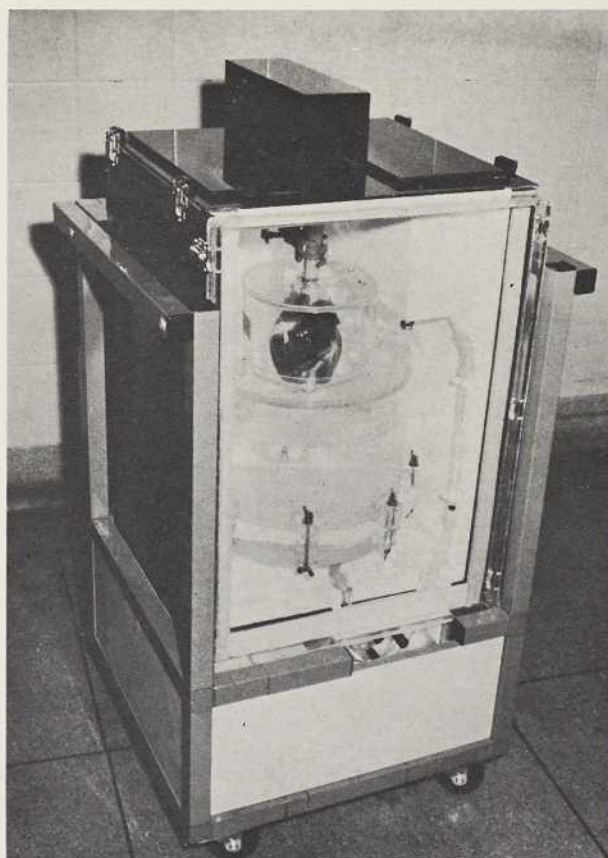
Figure 2 — Insulated portable container for transport of hearts (10 hour travelling capacity). Contains 350 g. greyhound heart. Cooling blocks of 10% potassium chloride maintain temperature of 5°C, and battery drives perfusion pump. Gas cylinder at rear. Proposed basic module for « heart-bank » system (see text).
