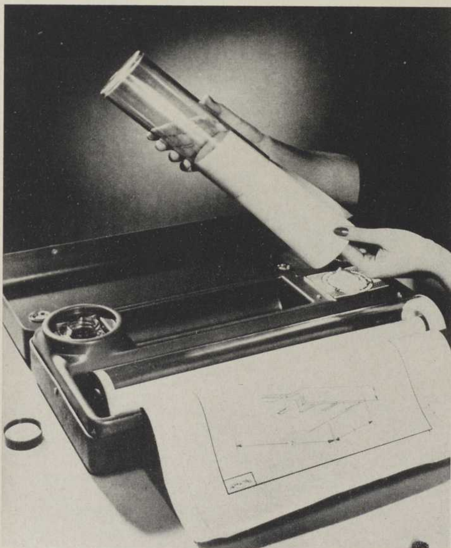
Portable Printer makes reproductions of everything from pencil drawings to typed or printed matter. The five and one-half pound unit requires a 110-volt electrical outlet and can be adapted for use in automobiles, boats or planes. Copy and paper are placed in a butyrate plastic tube and exposed to a fluorescent lamp. (PELprinter, Inc., 555 Central Ave., Orange, N.J.)
