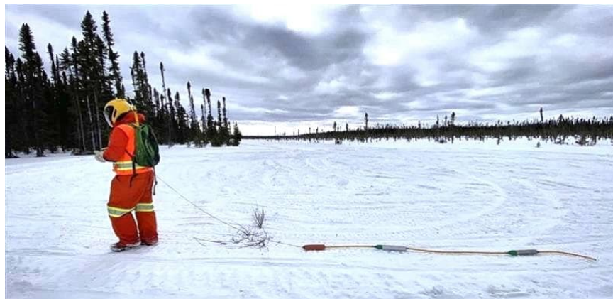
Photo D.3 — Ground penetrating radar (GPR) survey equipment – 12.5 MHz antenna
