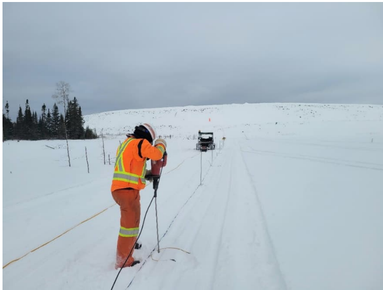
Photo D.1 — Electrical resistivity tomography (ERT) survey equipment
