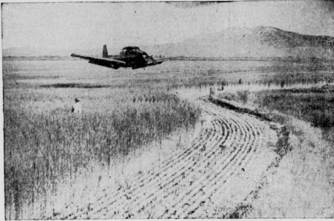
Making a pass at 30-foot altitude over a farm in the Fairfield Valley of Idaho, this light plane churns the air to keep frost from condensing on the wheat crop below. This was one of six planes that took part in a successful experiment to keep frost from killing the crops in the 5,000-foot-high valley.
