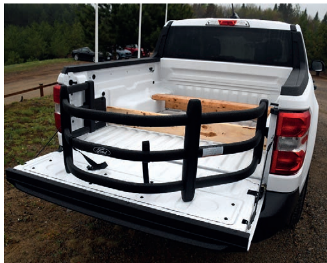
A wide range of accessories can be added to the cargo bed, such as these rails that extend the loading surface and keep materials more secure.
