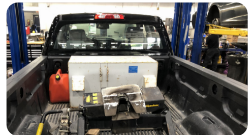
Example of a vehicle with a fifth wheel trailer hitch
