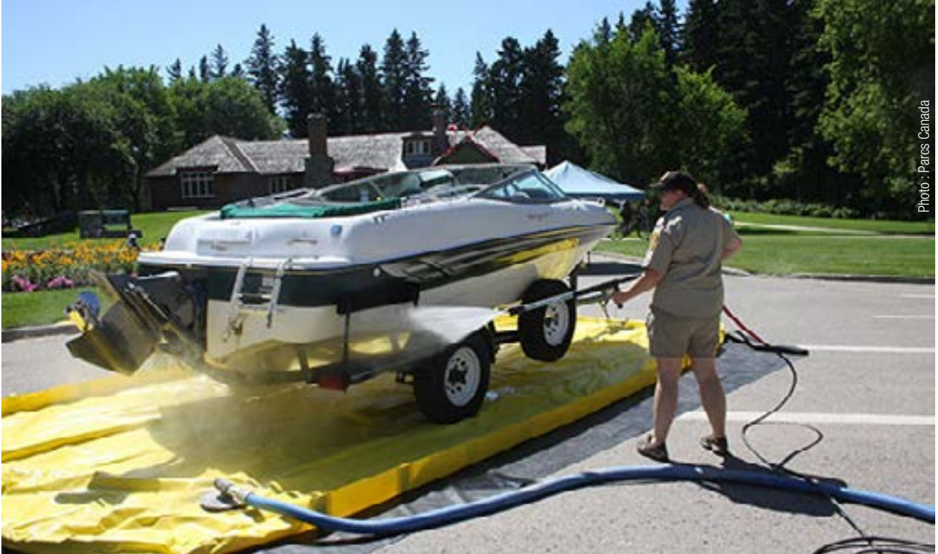
Use of a membrane to recover waste water from a watercraft decontamination station © Parcs Canada
