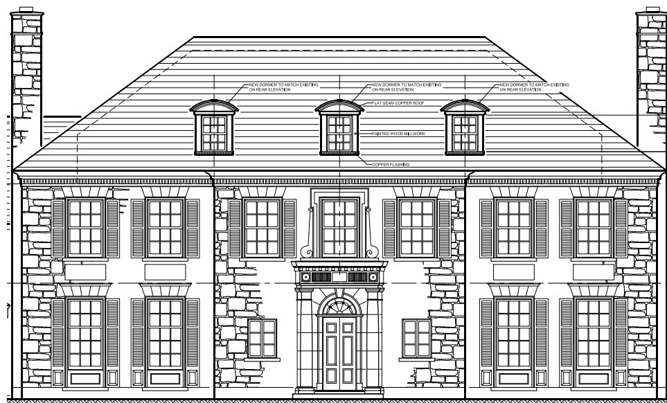
Detail of artistic rendering shown at the hearing illustrates the proposed front dormers at 3122 Daulac. The garage has been omitted.
