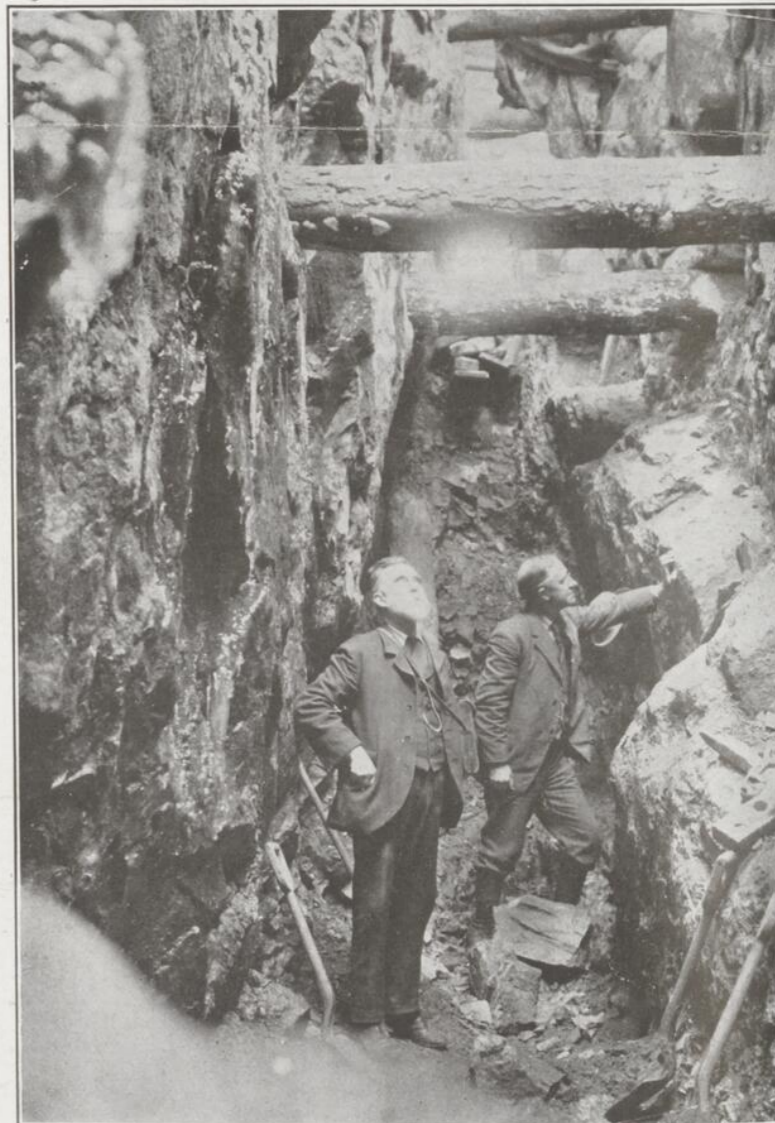
CANADA'S RICHEST SILVER POCKET—Dr. Robert Bell, late chief geologist of Canada, and Mr. Wm. C. Hidden, inspecting vein No. 49 of the Nipissing Mine. The vein is from 20 to 28 inches wide and about 17 feet deep, and has averaged about 8,000 ounces of silver to the ton. From the pocket shown in the illustration $624,000 worth of silver has been taken. This pocket is the one that caused all the talk in the Guggenheimer negotiations.
