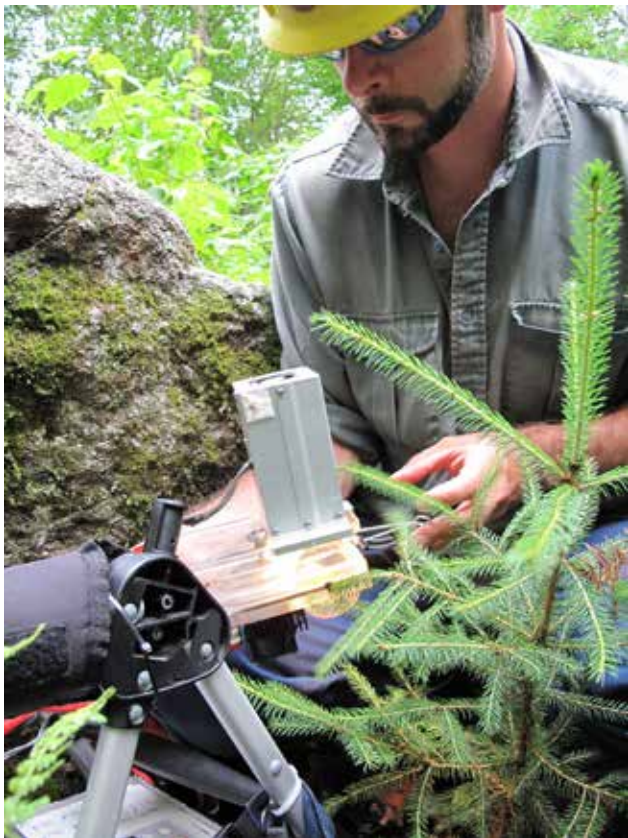
Figure 26. Gas exchange measurements (including photosynthesis) on a planted red spruce seedling. Photo : Daniel Dumais.
