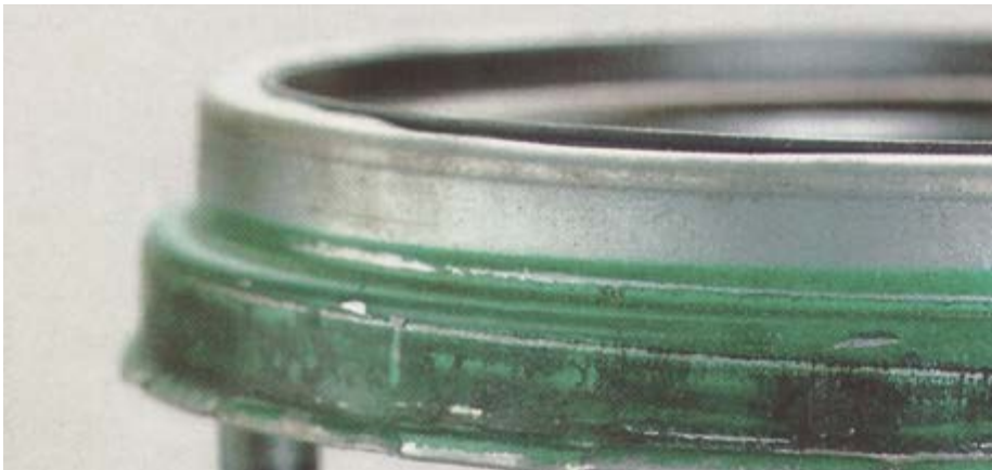
Figure 8 Distortion of the metal casing caused by the use of improper tools
