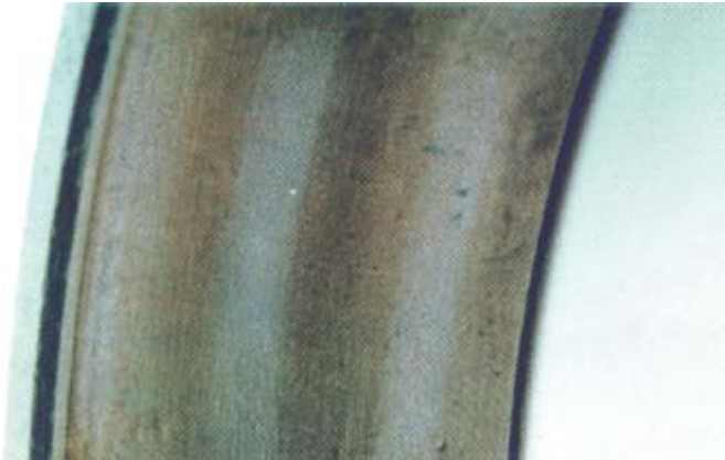
Figure 6 Premature wear of the inner race of a bearing caused by an overly tightened adjustment
