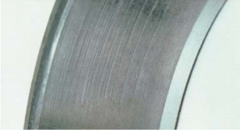
Figure 1 Pieces of metal or grit in the lubricant
