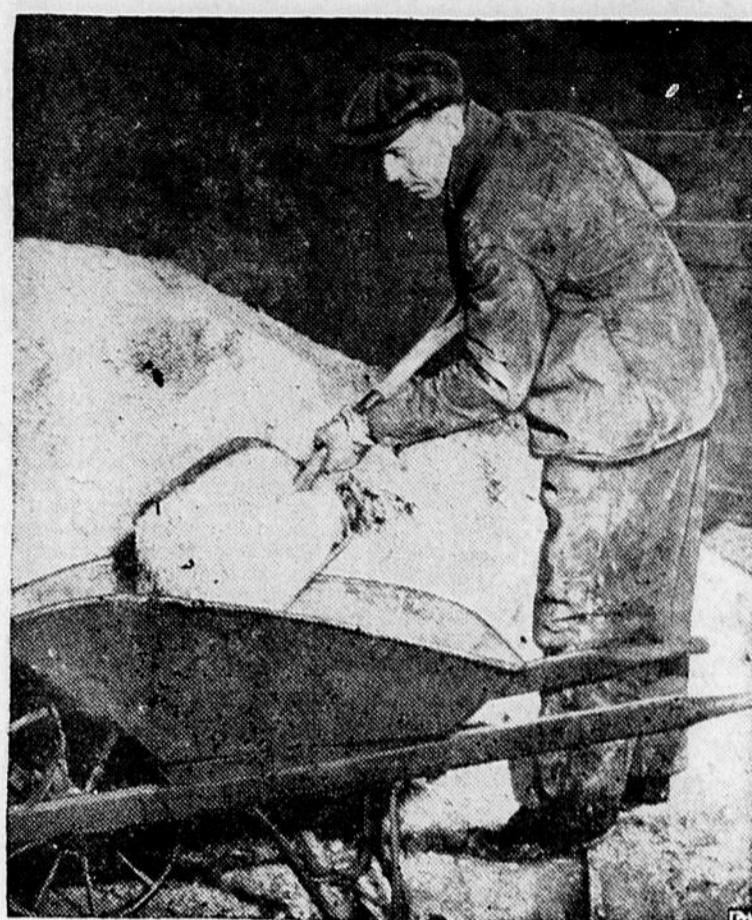
Salvaged glass is nearly 100 per cent reclaimable. Here a workman shovels salvaged glass that has been ground into powder. Melted to a white heat in a roaring furnace, it will go to ingenious machines that mould it into useful articles.
