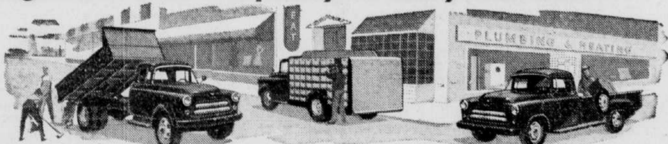
"H" model Chassis and Cab with Dump Body—12,000 lbs. G.V.W. "F" model Chassis and Cab with Bottler's Body—15,000 lbs. G.V.W. "D" model Express—9-foot body, 126" wheelbase—8,800 lbs. G.V.W.
