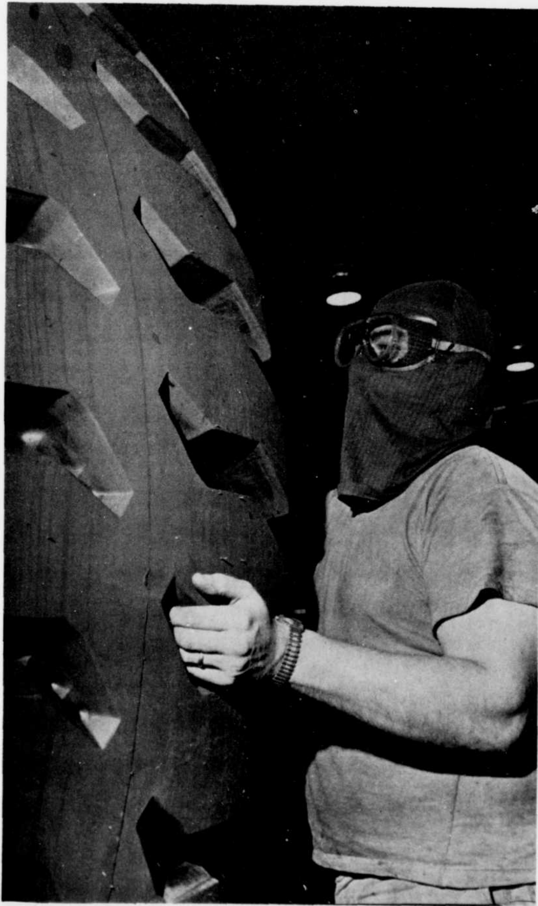
TIRES OF INDUSTRY — Protected against flying particles, employee at Goodyear's Valleyfield, Que., plant prepares to grind mold overflow from earthmover tire, the largest made in Canada by Goodyear. It is
