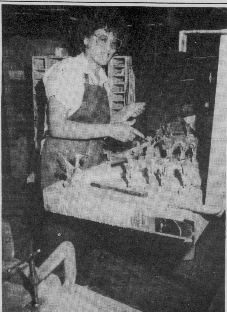
Guitabec craftswoman Guylaine Brochu poses wooden laths to the inside of the guitar face. The positioning of the laths are what gives each guitar its particular sound.
