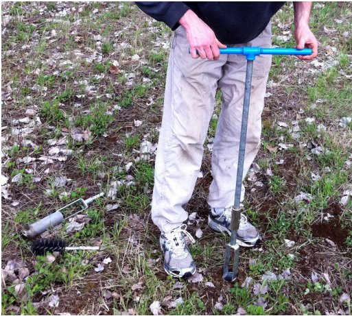
(a) Drilling a hole with a 5 cm hand auger
