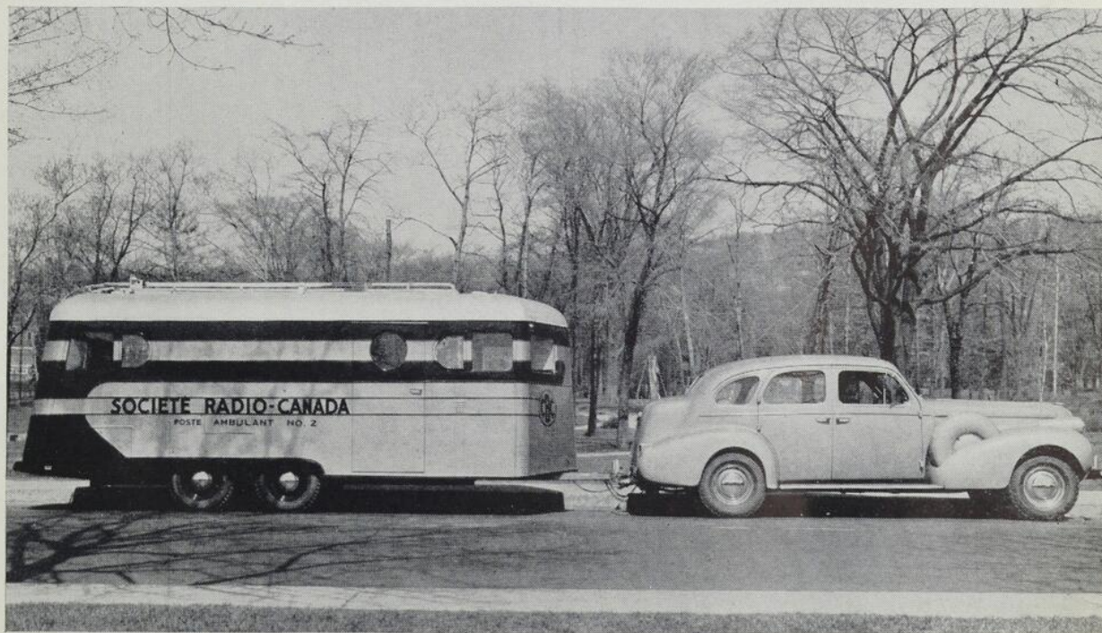
Mobile recording and shortwave transmitting and receiving unit of the Canadian Broadcasting Corporation.
