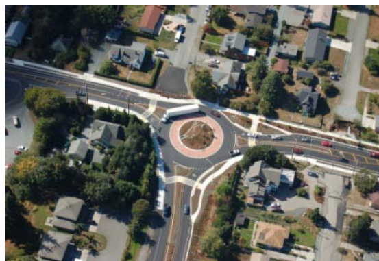
Figure 8 A single-lane roundabout
